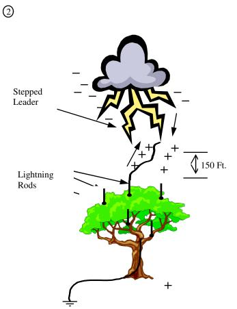
In a lightning protection system, the positive ground charge is attracted upward through the conducting cables attached to the tree. When the negative downward stroke from the cloud is about 150 feet above the top of the protected tree, the positive ground charge leaps upward to meet the lightning bolt.
