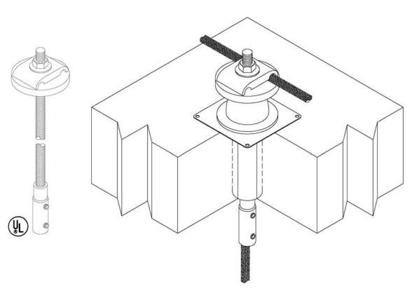
597C Thru Roof Connector for 1-1/2" PVC
